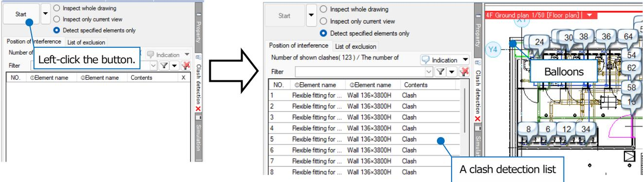
The number appears on the clashing position in the drawing works in a ganged manner with the listing number in a clash detection panel.
