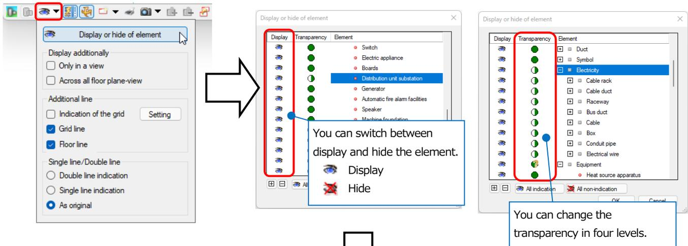
Left-click [Transparency of CG display of [Around-view]] to change between [Nontransparent], [Semitransparent], or [Transparent] for the element set up by [Display or hide of element].
