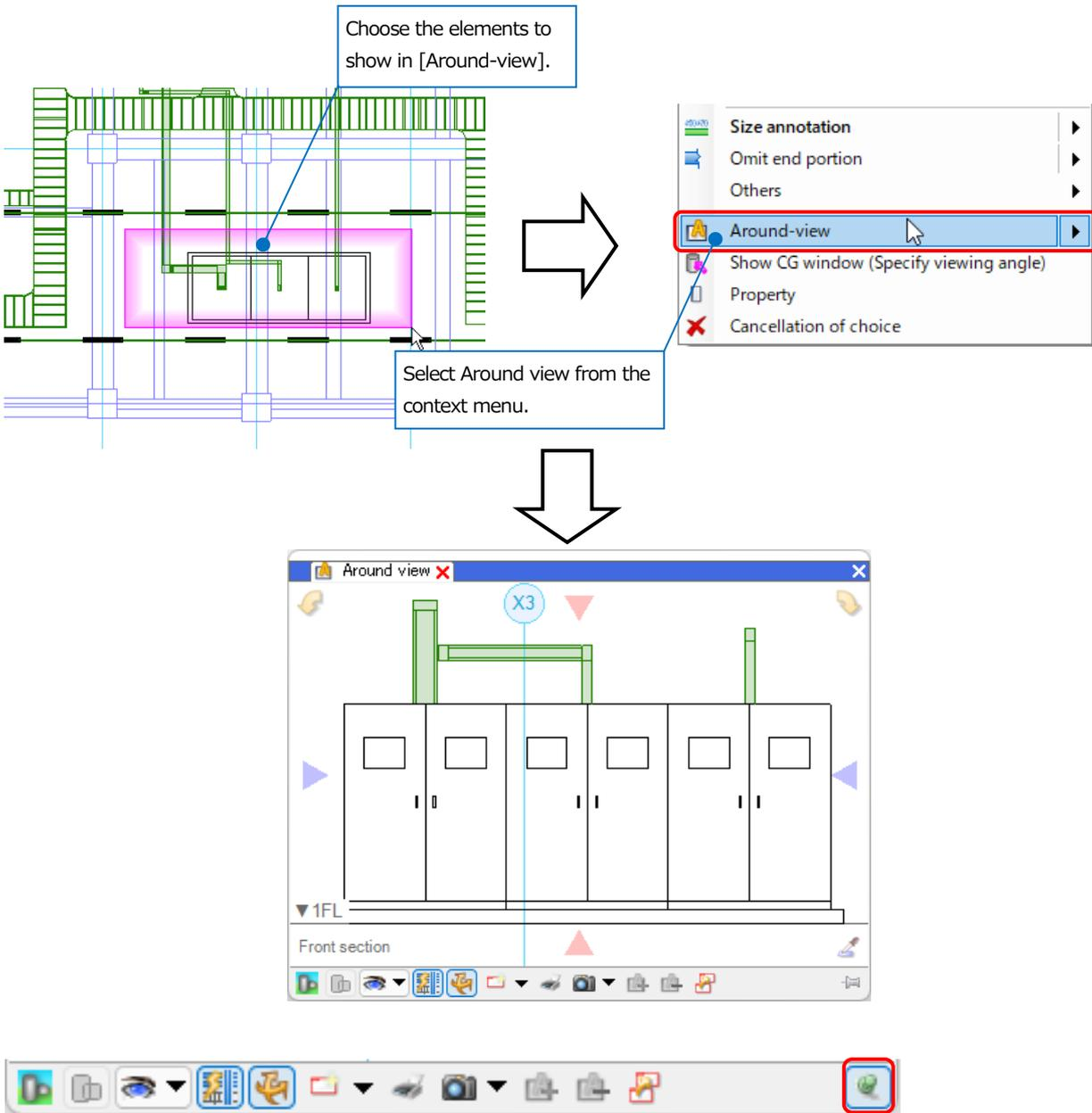
You can activate up to ten around-views at the same time. When you stick up the pushpin in an around-view, the around-view is kept alive and you can open the next around-view that will be activated in another window. When you lay down the pushpin, you can update the elements shown in the same window.
