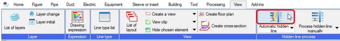
You can set target elements of hidden line process, or hidden line types by [Setting of automatic hidden line].
