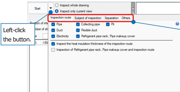
Numbers appear at the clashing position between the Inspection routes or the Inspection route and the Subject of inspections. A balloon appears on the drawing to show the number.
