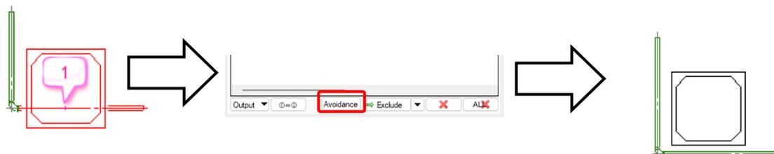
If the clash elements are beams and pipes, beams and rectangular ducts, or beams and spiral ducts, Rebro adjusts the route height to avoid clashes.
