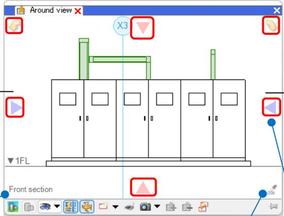
Specify the direction to show. Select "Angle appointment" to specify the azimuth angle and elevation angle optionally.
