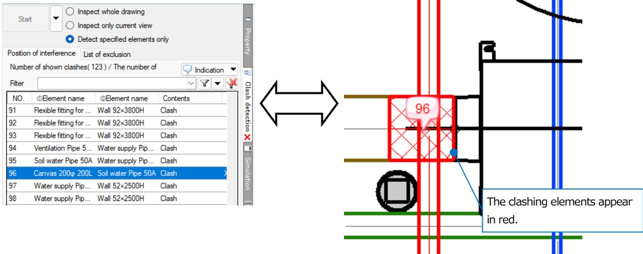
Double-click the balloon on the drawing or the number in the panel to start CG screen, where you can check the clashing point.
