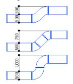
S pipe is applied for the gap width in the case of L≥D+H
