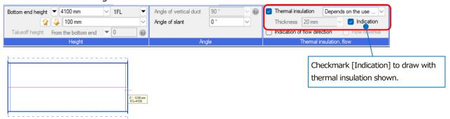
When you select "Depends on the use settings", Rebro reflects the thermal insulation thickness set for each use.
