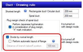
Checkmark "Divide by normal length" to show the flanges at the normal length that are set up in the material subsets.
